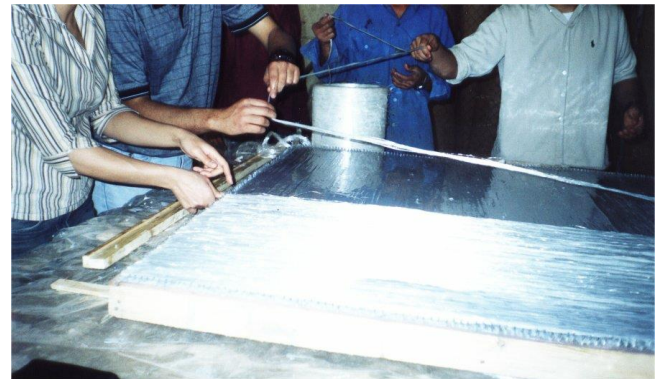
Figure 3A: Preparation of fibers into the mold (0° Fibers)
