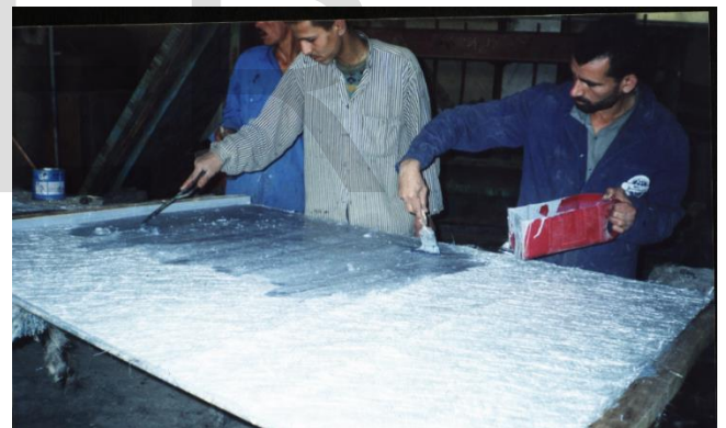
Figure 3C: Adding the polyester resin
