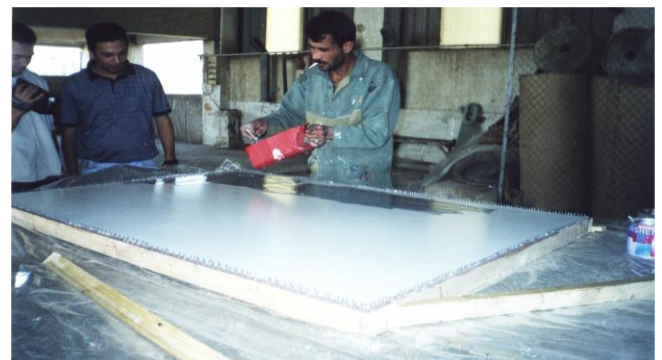
Figure 3D: Compacting the resin manually
